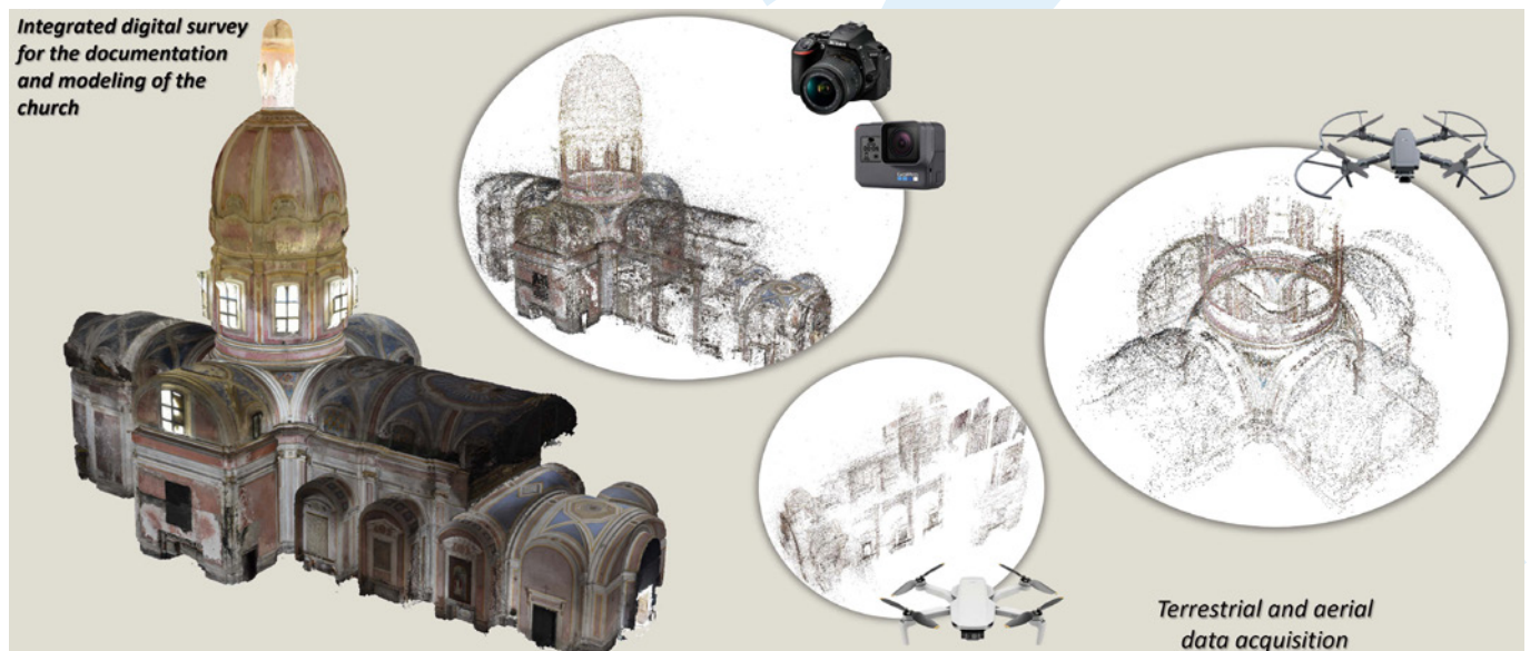
Fig. 3. Three-dimensional model of the Church of Santa Maria della Vita obtained from terrestrial and aerial photogrammetric survey (processed by R. Iaderosa and D. Iovane).
